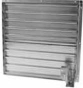
This damper has a flanged frame and is designed to fit the inside flanges of the optional wall housing or wall mounting collar. The frame and blades are constructed of galvanized steel and are rated to 3000 FPM with proper clearance as provided by all factory accessories. The damper body recesses into the opening for a flush appearance.
