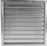
This damper can greatly reduce the infiltration of outside air and although not completely watertight, will provide weather protection in an economical fashion. Constructed with a galvanized frame and aluminum blades this damper is rated to 2000 FPM with the proper clearance as provided by all factory accessories. The damper body is recessed into the opening for a flush appearance.
