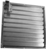
The motorized option improves weather protection by providing a tighter closure seal and is recommended for all supply applications. Heavy-duty dampers are constructed with galvanized frames and blades and are rated to 3000 FPM. The damper body is not recessed providing extra clearance between the fan and damper blades.
